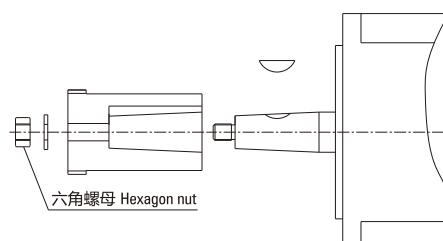
电机轴为锥形轴且带螺栓 The motor shaft is a conical shaft and is provided with a bolt
