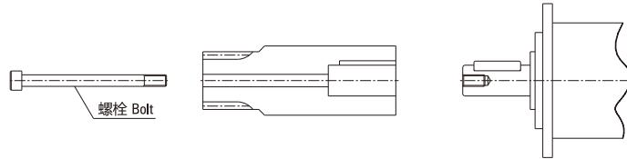
( 锥轴: 伺服马达轴有螺栓 Cone axis: Servo motor shaft with bolt )
