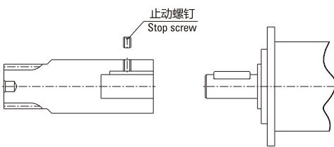
( 直轴: 伺服马达轴有螺孔 Direct-axis: Servo motor shaft with thread )
