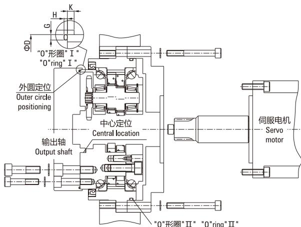
● 图C.2: 装配密封 Figure C.2: Assembly seal
