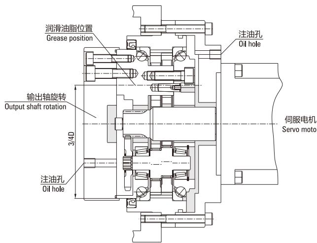
● 图C.10: 润滑油注入位置(垂直) Figure C.10: Lubricating oil injection position (Vertical)
