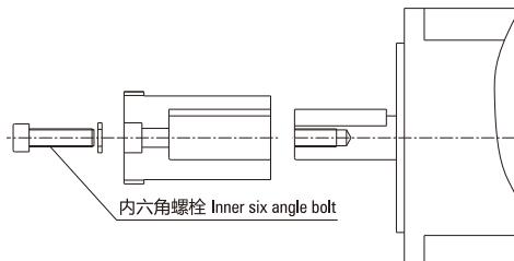
电机轴有螺孔 The motor shaft with a screw hole
