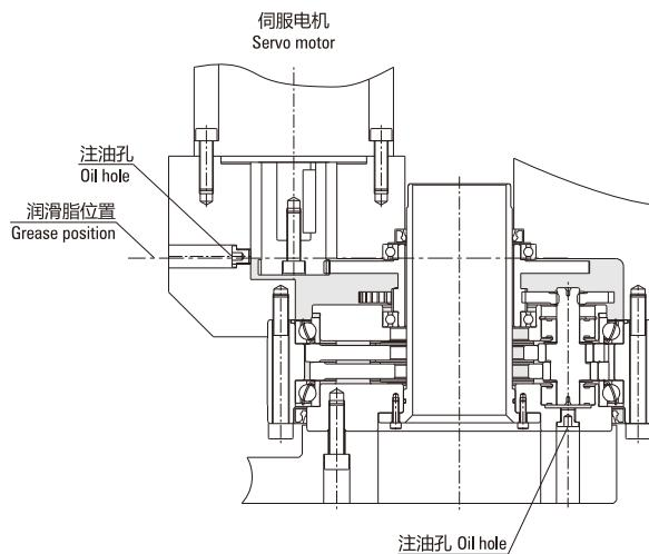
(安装垂直轴-2 Install vertical axis-2)
