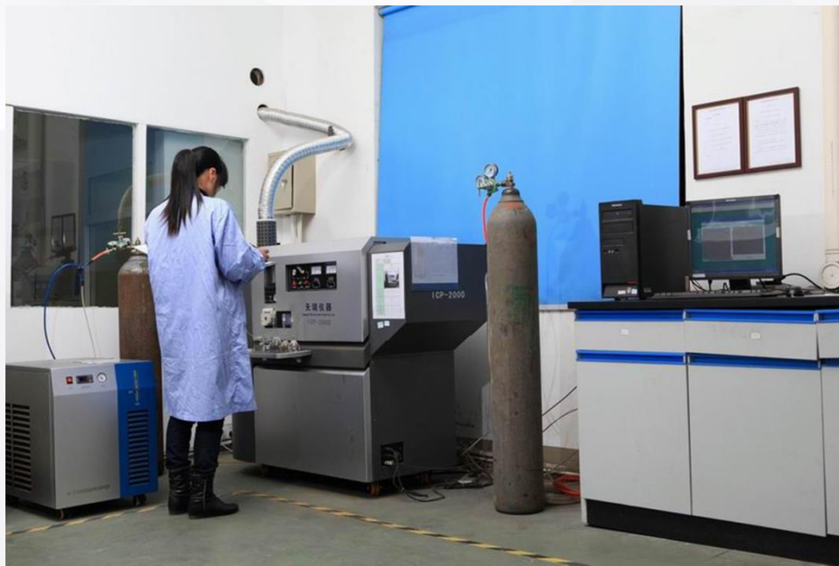
ICP Tester: Testing the internal ingredients of raw materials
